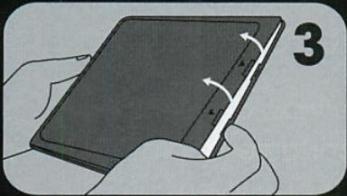
**Separate the hard plastic case by locating the indicated arrows and unhinging each snap on all four sides of the case**
