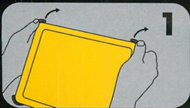
**Release corners and remove shield stand**
