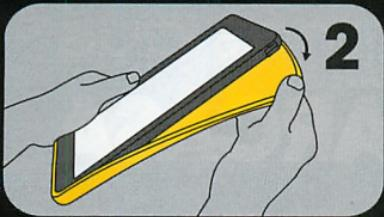
**Peel away and remove the outer silicone casing**
