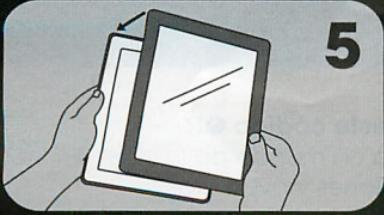
**Place the lid on top of the device and snap the two halves together, locking the device in place**
